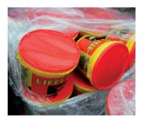
Damaged buckets caused by the placing and removal of a top pallet.
